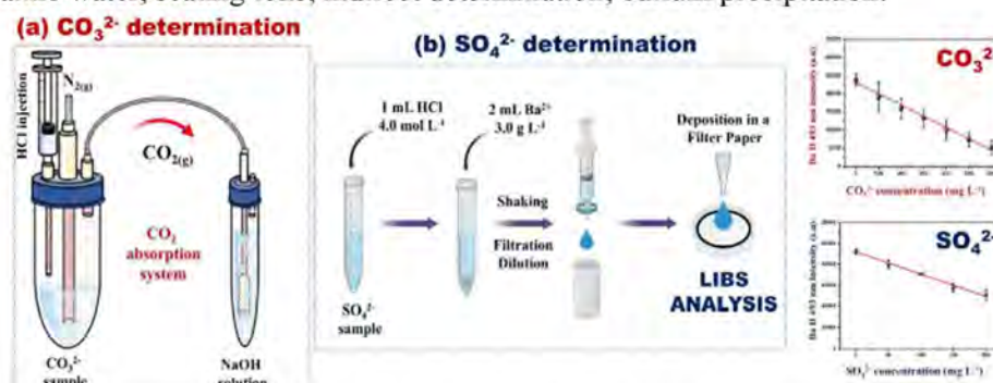
Fig. 1 (a) \text{CO}_2 absorption system for \text{CO}_3^{2-} determination and (b) analytical method for \text{SO}_4^{2-} determination.
