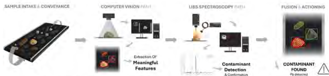
Fig. 1 LIBS assisted by Computer Vision workflow for real-time contaminant detection.
